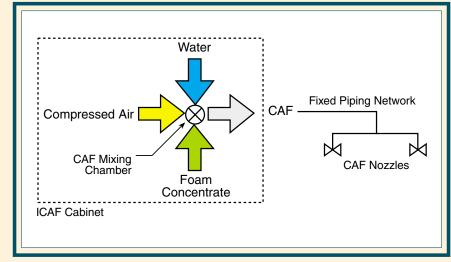
Figure 1. Schematic of a CAF system
