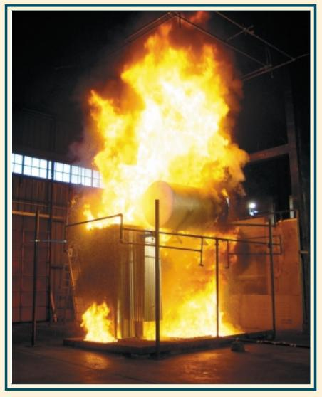
Figure 4. Fully developed transformer fire
