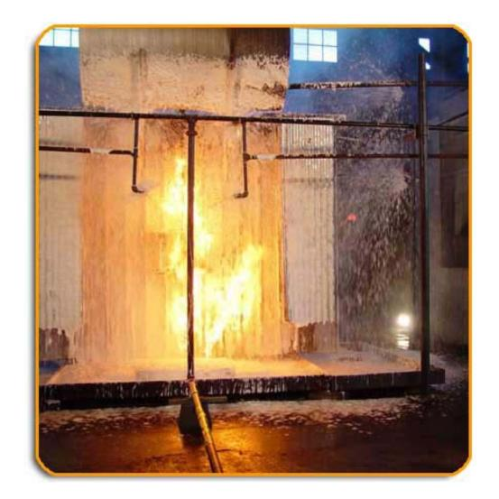
FireFlex's CAF-based system controlled a simulated power transformer fire in less than 45 seconds and fully extinguished the blaze in under 1.5 minutes. A traditional "deluge" type uses up to 10 times the water flow and is capable of extinguishing transformer fires in approximately 4 minutes. This tremendous water usage creates a large amount of hazardous waste caused by water mixing with contaminants from the transformer.
