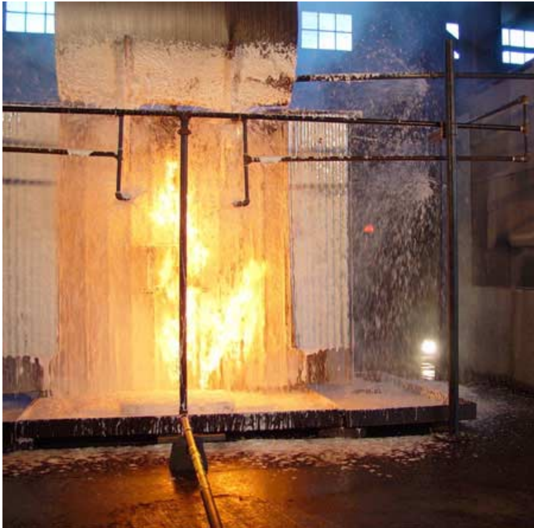
Compressed air foam, based on NRC-IRC patents, extinguishes a transformer fire
