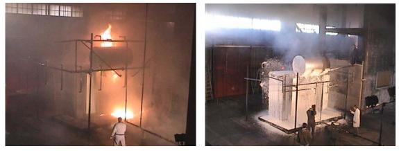
Figure 6 – Water Spray system vs CAF system for power transformer protection
