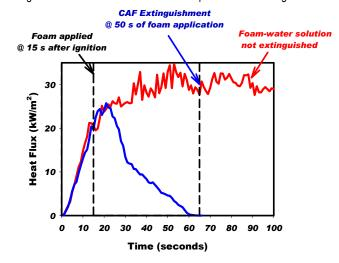
Figure 4 - Heat Flux with CAF and Foam-Water Solution Extinguishment
