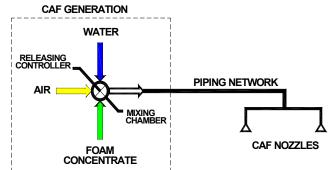
Figure 1 – Schematic of a CAF System
