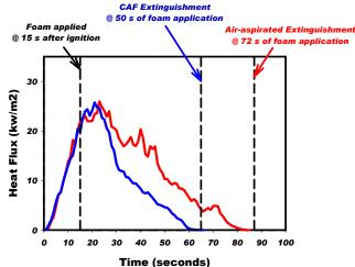
Figure 3 - Heat Flux with CAF and Air-Aspirated Foam Extinguishment
